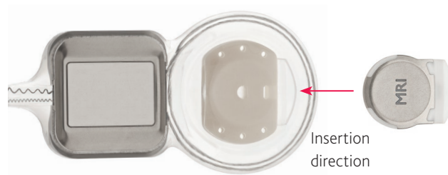
Figure 22: Non-magnetic cassette insertion direction
