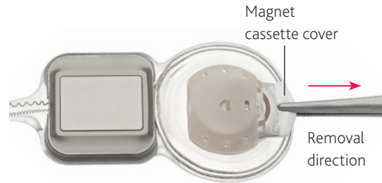
Figure 19: CI624 implant with magnet cassette partially removed
