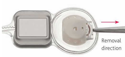
Figure 21: CI624 implant, magnet cassette removal using metal tab
