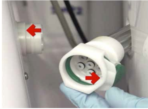
Figure 8: Ventilator Lines Connection Port
