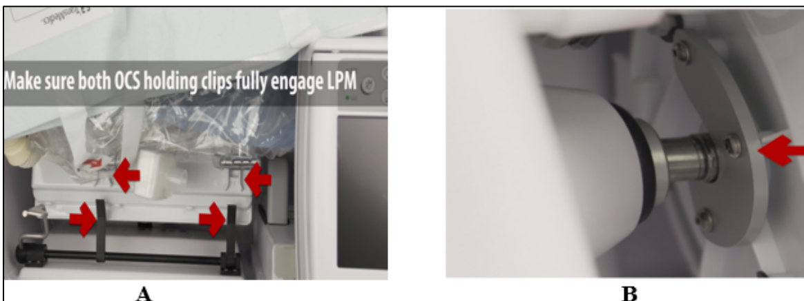
Figure 7: Holding Clips Engaging with the LPM (A) and Ventilator Actuator Engaged with the Bellows Plate of the LPM (B)
