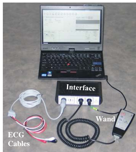
Figure 3 – The OMNI II Programmer consists of a battery-operated laptop computer that runs the OMNI SMART Programmer Application Software connected to an OMNI Programmer Interface and the OMNI Programmer Wand.
