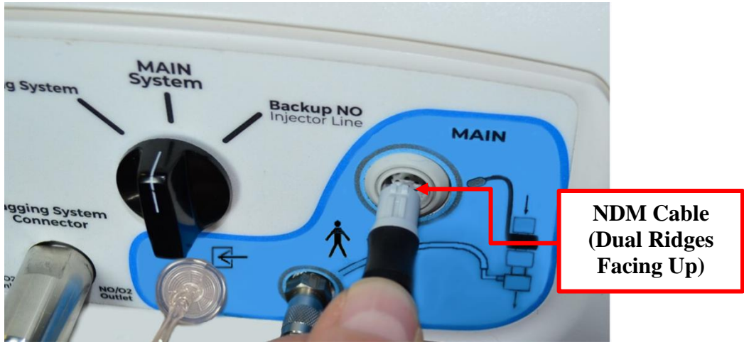
Figure 14: NDM Cable Orientation (dual ridges facing up)
