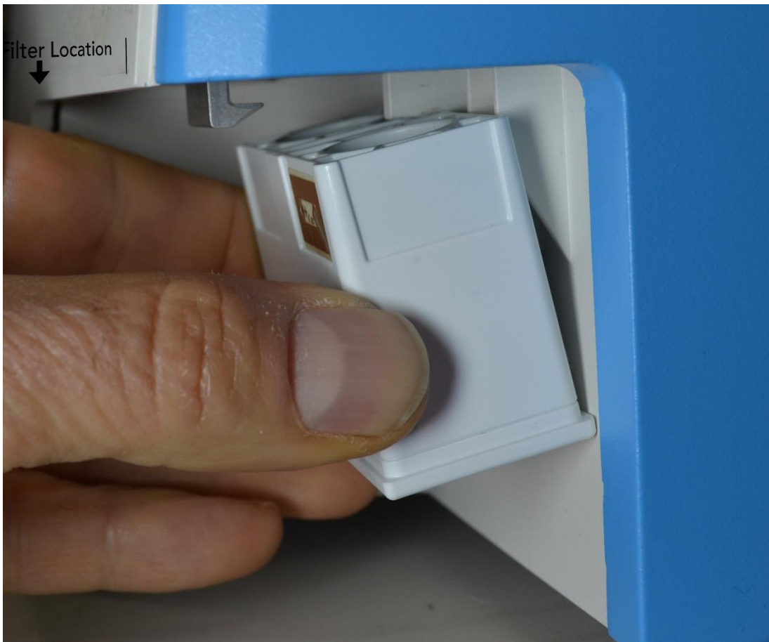
Figure 26: NO 2 Filter correctly aligned on the LungFit PH Filter Insertion Guide. At this point, sliding the filter vertically will align the filter openings with the LungFit PH fittings and result in a successful filter installation, which is evident when the filter is clicked into place.
