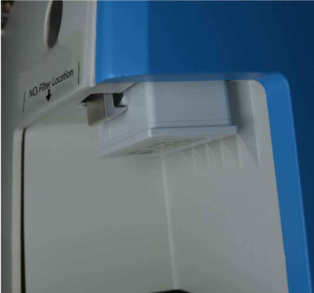
Figure 27: NO 2 Filter Successfully Installed and Locked in Place.
