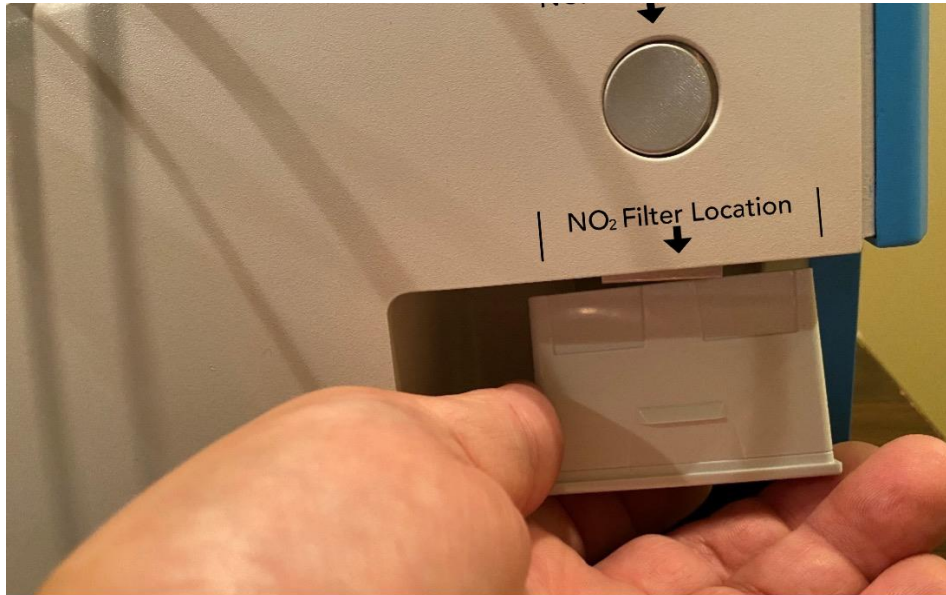
Figure 24: New NO 2 Filter lined up and ready to be slid in vertically
