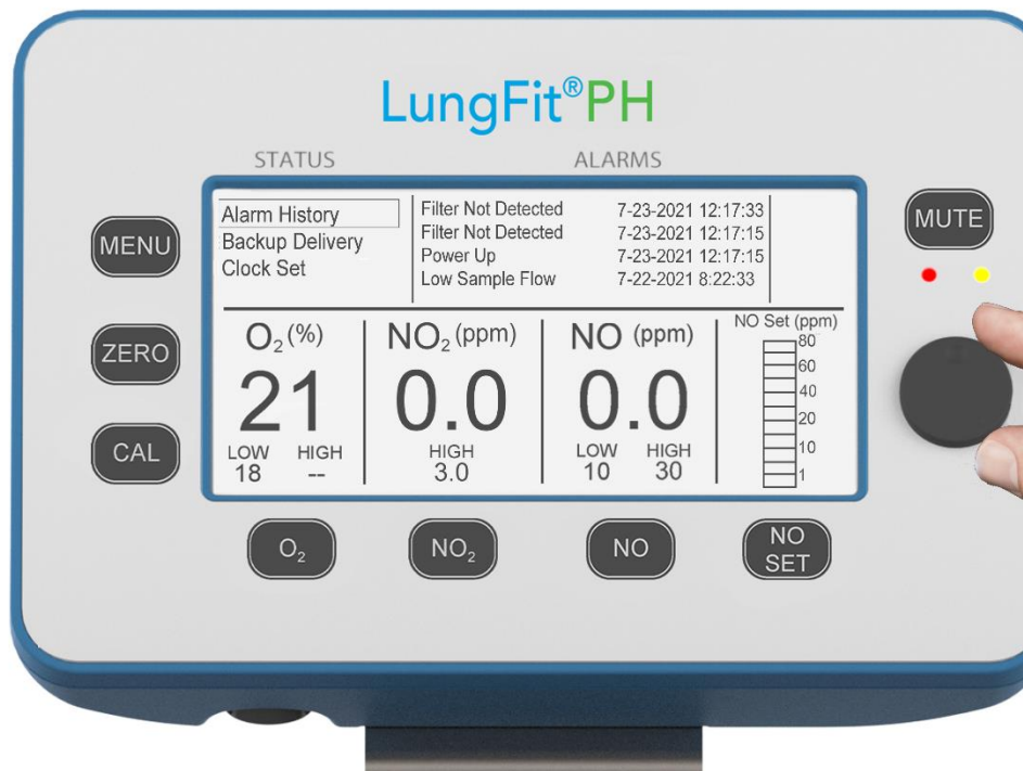
Figure 35: Alarm History Screen
