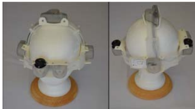
Figure 3. BrainPulse headset viewed from the front (left panel) and from the right (right panel).
