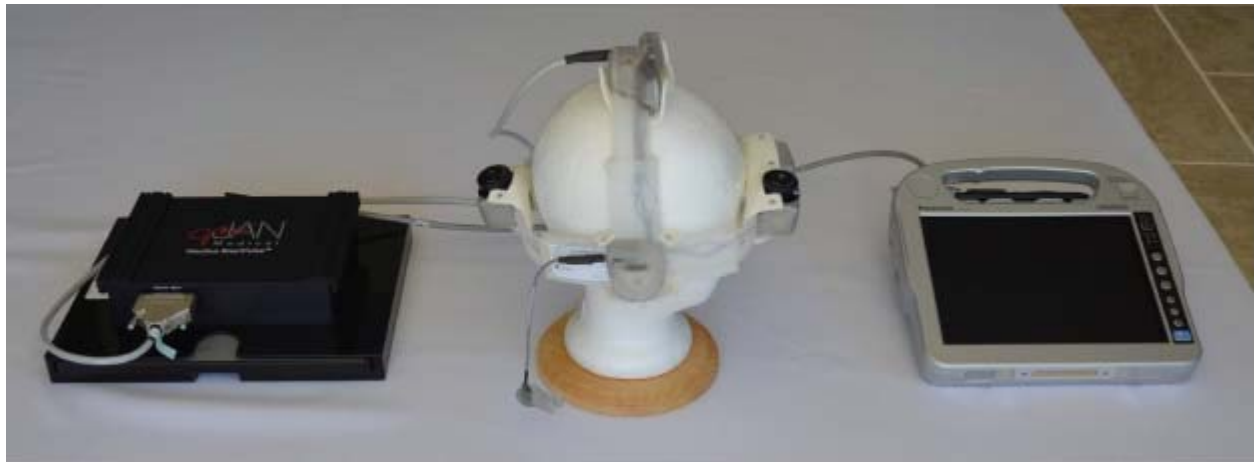
Figure 1. BrainPulse system consisting of the data collector and battery, headset containing sensors, and computer.
