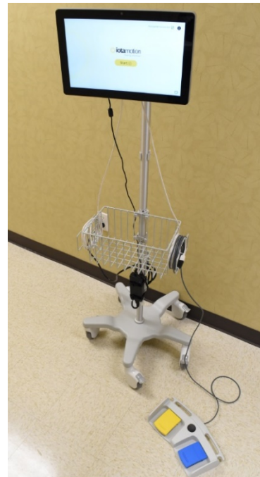
Figure 6: iotaSOFT | Control console, footpedal, rolling stand assembly with power supply and USB cable extenders.
