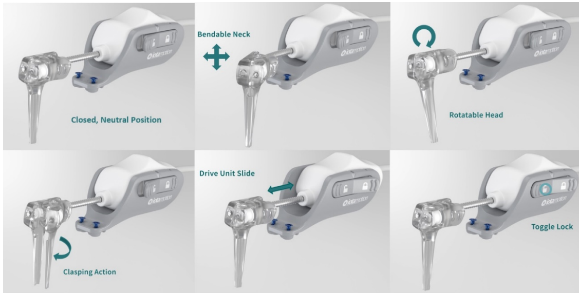
Figure 3: iotaSOFT™ | DRIVE Unit adjustability features to manually manipulate drive head position and electrode array insertion trajectory.
