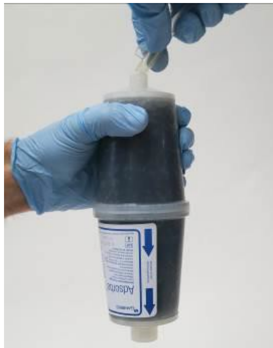
Figure 15a: Installing the Solvent Removal Column (bottom first)
