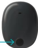
**Note:** If you press the power button on the smart transmitter and no LED appears, press and hold the power button for about 5 seconds to turn it on.
