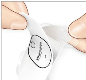
2. Align the smart transmitter over the sticky side (center) of patch and press firmly to secure.
