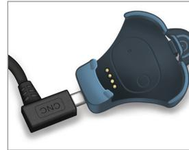
**3. Line up the four gold pins on the bottom of the smart transmitter with the four gold pins on the charging cradle.**
