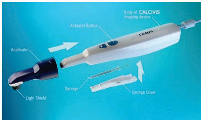
Figure 8. The CALCIVIS imaging system consists of a specialized intra-oral camera capable of imaging very low level, transient luminescence when a calcium-activated photoprotein is applied to enamel surfaces of teeth.
