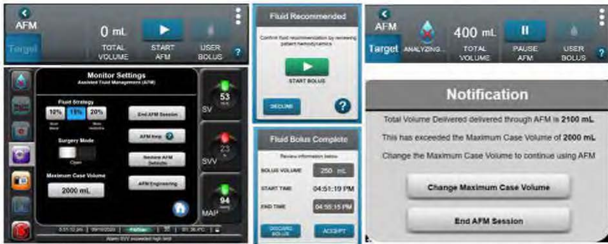
Figure 1: The AFM dashboard before AFM is started (top, left); an example of the AFM Settings Screen (bottom, left); the fluid delivery recommendation pop up (top, center); an example of information on fluid bolus delivered by the user (bottom, center); an example of the AFM dashboard while AFM is running (top, right); an example of notification prompting the user to either change the Maximum Case Volume or End AFM Session (bottom, right).
