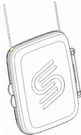
Figure 11.6 eCLS with two leads connected enclosed in case.
