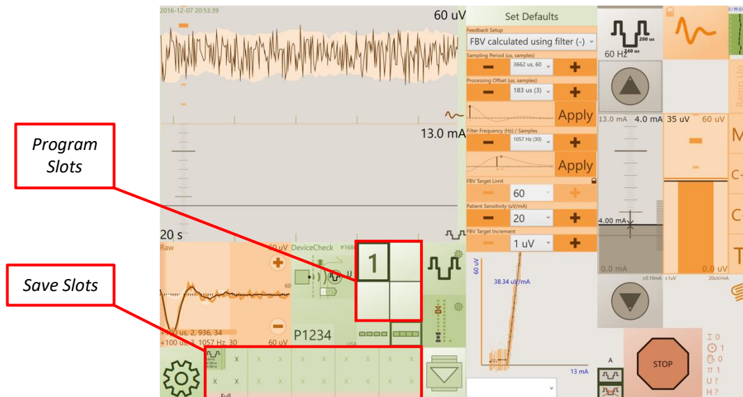
Figure 6.22: Location of the program slots and save slots on the CPA.
