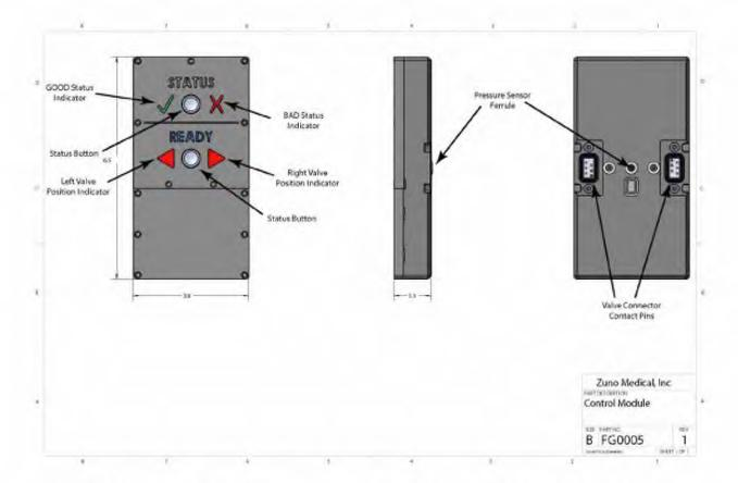
The device is composed of 3 primary components: the lid assembly (which includes the valves and has a space for attaching the control module), the base assembly (which houses the instruments to be sterilized), and the control module (which electronically controls valve actuation and monitors the low-pressure state of the container).
