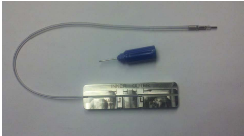
Figure 7: Pre-loaded Tool with Repair Lead Section and Torque Wrench
