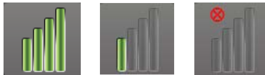
Figure 8: Link Quality Indicator (Excellent, Poor, No Link)
