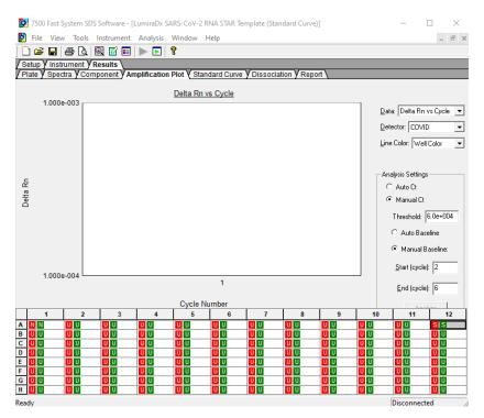
8. Select the 'Amplification Plot' tab then select 'COVID' from the 'Detector' drop-down menu in the top right corner and select the 'Manual Ct' box. In the 'Analysis Settings' window define 'Threshold' as "6.0e+004". In the 'Manual Baseline' window set the 'Start (cycle)' to '2' and set the 'End (cycle)' to '6'.
