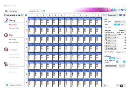
Select just well 'A1' and re-set 'Well Type' to 'NTC' (No Template Control) from the drop-down menu. Click the 'Name' button next to and define the 'Well Name' as "NEC"(Negative Extraction Control). Select just well 'A12' and re-set 'Well Type' to 'Standard' from the drop-down menu. Click the 'Name' button next to and define the 'Well Name' as "PEC" (Positive Extraction Control). The other wells will remain 'Unknown' unless defined as Samples Names (optional).
