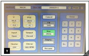
Note: Pausing a run will not cause depressurization of the vessel. The vessel will remain under pressure and serious injury can occur if the lid is removed while the vessel is under pressure.
