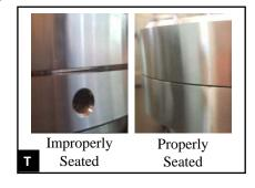
b. Position the locking rings over the lidded vessel as shown in image U below. If the lid is seated properly, the locking rings will slide onto the lid easily.
