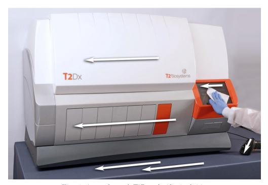
Figure 1. Areas to clean on the T2Dx and unidirectional wiping.
