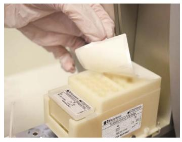
Figure 3. Remove top seal.
