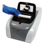
NOTE: If pouch does not slide into the instrument easily, gently push the lid of the instrument back to ensure that it is completely open.
