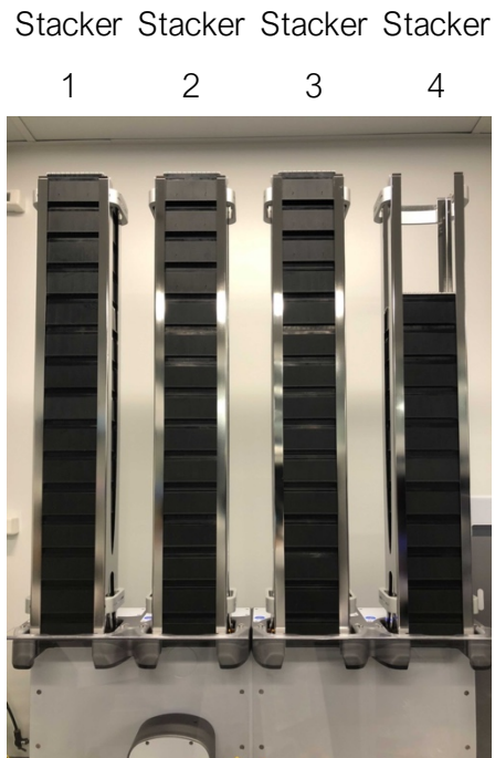
Figure 7: BenchCel4 Stackers use pipette tips starting from right to left. Stacker 4, which holds a maximum of 11 boxes, is used first.
