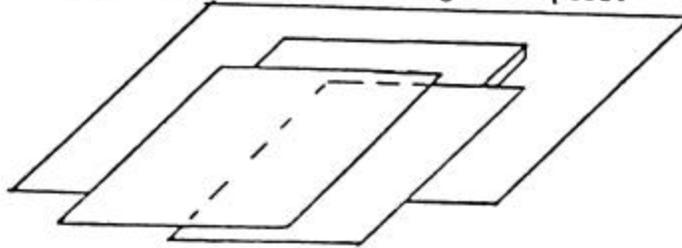
c) Slide assembly, grid side down, positioned over the plastic cassettes.
