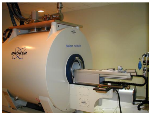
Preclinical MRI machine - one of the pieces of equipment used in the NCTR Bio-Imaging Facility.
