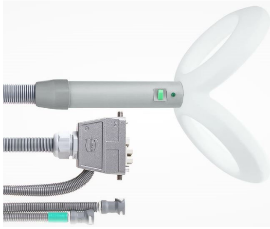
Fig.1 Double Cone Coil for magnetic stimulator
