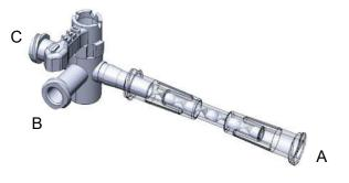
6. Turn the flow diverter "Off" arrow of the mixing manifold towards luer port "C" of the mixing manifold then prime the mixing manifold by filling the fluid path (up to luer port "B" of the mixing manifold) with premixed Lava<sup>™</sup>.
