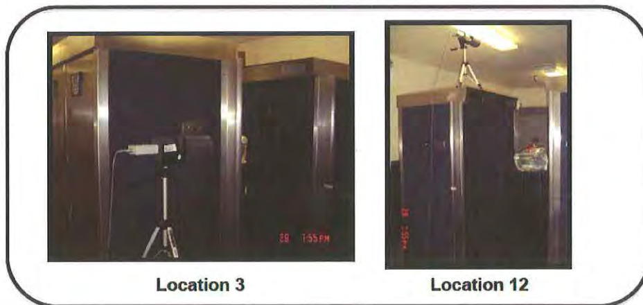
Figure 8-9. Ion Chamber at Location 3 and 12 During Area Survey
