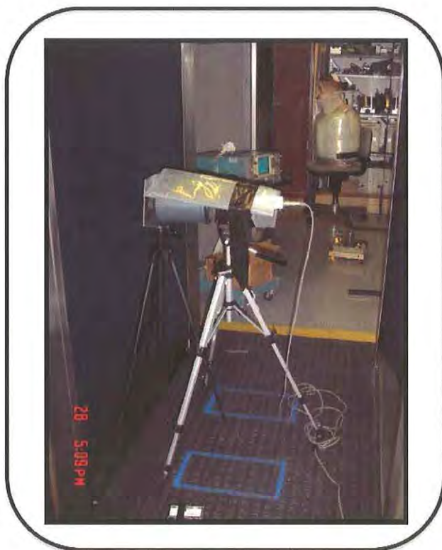
Figure 8-3. Ion Chamber Configuration for HVL Readings
