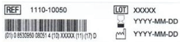
Figure 2. Peelable Device Label (Triplicate) With UDI
