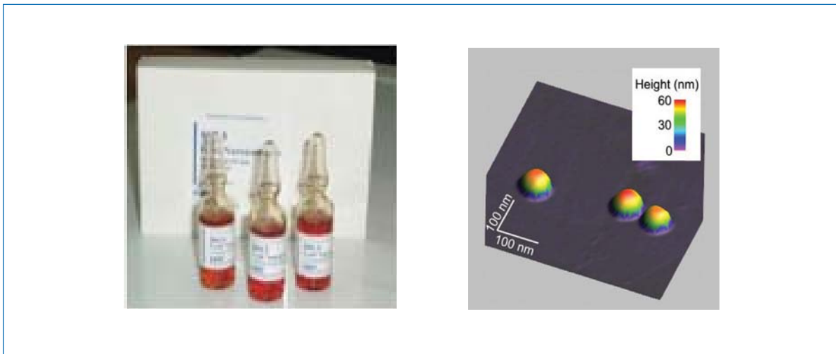
Figure 2-2. (Left) NIST gold nanoparticle reference materials (RMs) 8011–8013. (Right) Atomic force microscopy image of 60 nm gold reference material nanoparticles.
