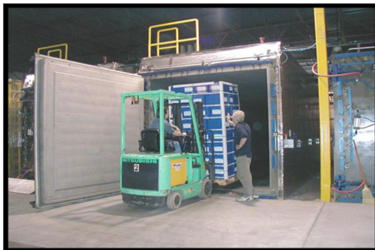
Figure 7: A Sterilization Chamber (Photo courtesy of Sterigenics)
