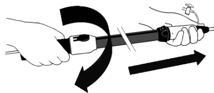
Figure 9. Actuating the device using mechanical advantage
