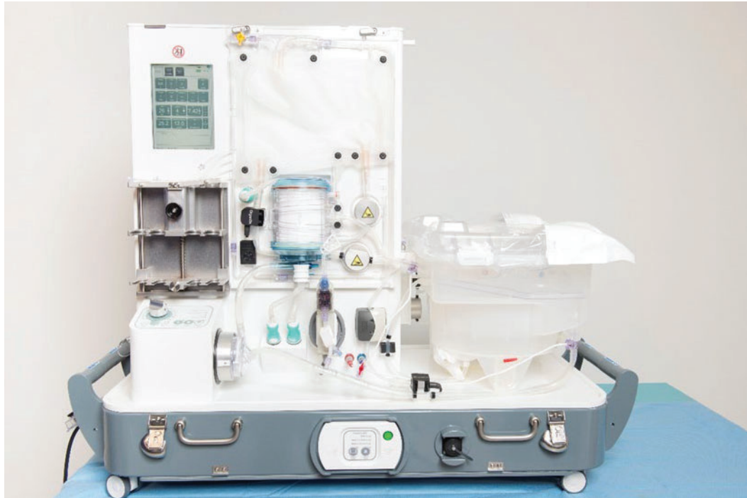
Figure 1: Components of the OrganOx metra® System. The figure shows the Liver Perfusion Circuit (Disposable Set) mounted on the Retained Unit
