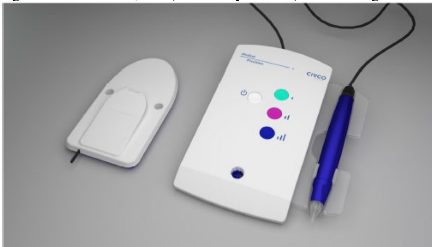
Figure 1: Control unit, Pen (with safety needles) and docking station
