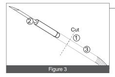
After the TransLoc electrodes have been implanted into the diaphragm and tunneled through the skin, the external end of the electrodes requires preparation before it can be connected to the FrictionLoc connector. The suture (1) between the tunneling needle (2) and the conductive pin (3) must be cut.
