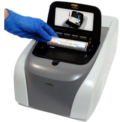
**Note**—The instrument lid must be opened completely. If the pouch cannot be easily inserted into the pouch chamber of the instrument, gently push the instrument lid back completely and try again.
