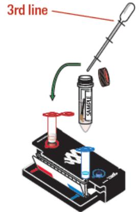
**NOTE:** *DO NOT use the transfer pipette to mix the sample once it has been added to the Sample Injection Vial.*
