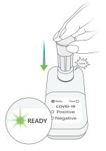
If Ready light is not blinking within 5 seconds, use palm of your hand to press down more firmly to start test.
