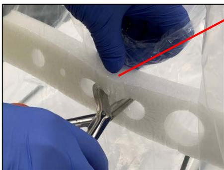
**Using scissors to cut between holes for a dual tubing circuit.**
