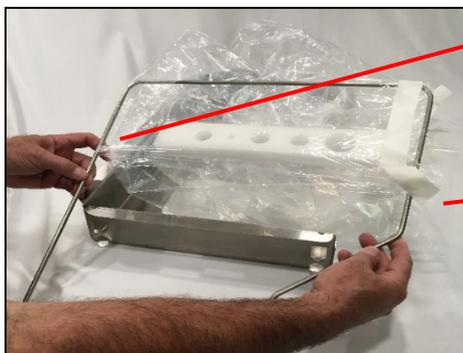
**Inserting rails into outer sleeve of the isolette.**
