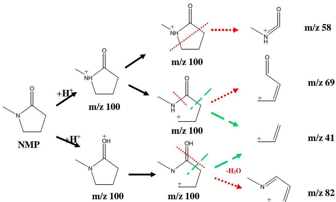
Note: For NMP ion transition of  $m/z$  100 $\rightarrow$ 58, there are two corresponding  $d_9$ -NMP transitions,  $m/z$  109 $\rightarrow$ 61 and  $m/z$  109 $\rightarrow$ 62. The transition of  $m/z$  109 $\rightarrow$ 62 was selected for the quantitation.
