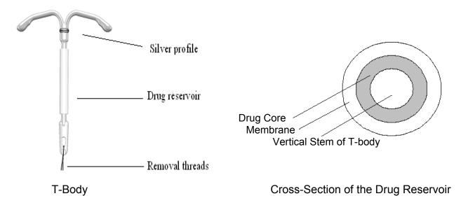
The T-body consists of a vertical stem with two horizontal arms. There is a loop with attached polyethylene removal threads at one end of the vertical stem and the two horizontal arms are at the other end. A silver ring is added around the top of the vertical stem of the T-frame to facilitate detection during an ultrasound examination. Other excipients in the LCS12 include silica colloidal anhydrous and barium sulfate.
