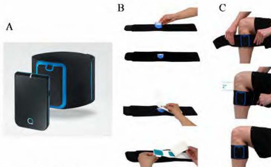
Figure 1. Quell-FM device and Band (A). Placement of device in Band and attachment of electrode (B). Placement of Quell-FM on upper calf (C).
