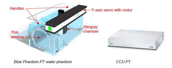
On the horizontal Y-rail, detector holders for various detectors can be mounted on a sliding shoe. The detector can be positioned in the Y-direction for measuring horizontal beams.
