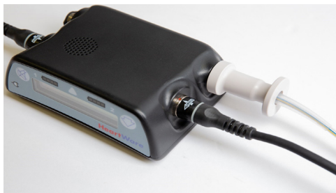
Figure 133: Driveline Cover completely covering Driveline Connector
