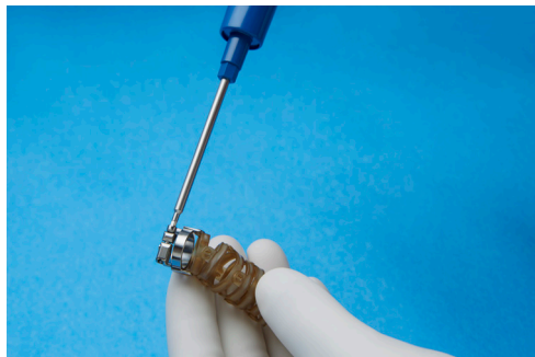
Figure 119: Loosen the strain relief clamp using the strain relief wrench
