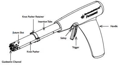
Figure 1. Permaseal<sup>™</sup> Delivery System
