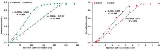
Figure 25: Linearity data for green and red fluorophores in areas of high and low illumination intensity. Signal normalized to the maximum output of the camera sensor. HII: high illumination intensity; LII: low illumination intensity; black dash lines: HII linear regression; black long-dash-dot lines: LII linear regression.
