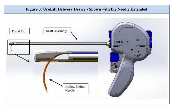
Figure 3. Details of the UroLift<sup>®</sup> Delivery Device, identifying the Distal Tip, The Shaft Assembly and, in a magnified view, the Hollow Nitinol Needle as it appears when protruding from the Distal Tip.
