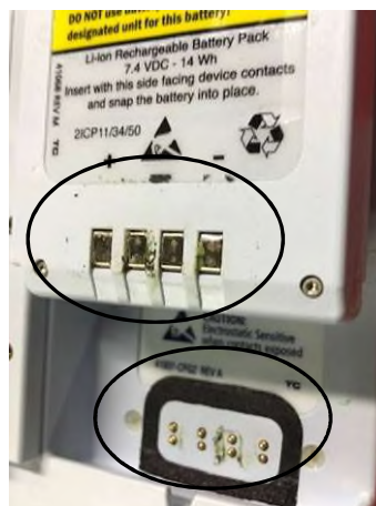
Unacceptable residue and corrosion buildup
