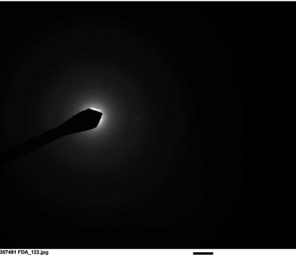
307491 FDA\_122.jpg Talc Ribbon Diff 15:28 6/16/2019 TEM Mode: Diffraction Microscopist **16:31** Camera: NANOSPRT5, Exposure: 800 (ms) x 5 drift frames, Gain: 1, Bin: 1 Gamma: 1.00, No Sharpening, Normal Contrast
