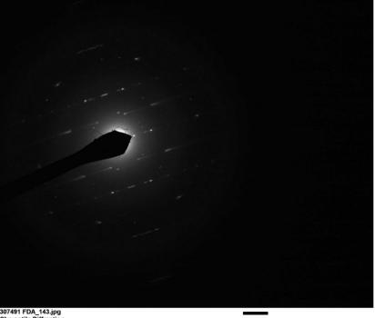
307491 FDA\_143.jpg Chrysotile Diffraction 15:51 6/20/2019 TEM Mode: Diffraction Microscopist: Camera: NANOSPRT5, Exposure: 800 (ms) x 5 drift frames, Gain: 1, Bin: 1 Gamma: 1.00, No Sharpening, Normal Contrast
