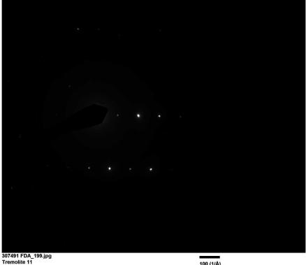
Tremolite 11 09:54 7/2/2019 TEM Mode: Diffraction Microscopist (0) Camera: NANOSPRT5, Exposure: 800 (ms) x 5 drift frames, Gain: 1, Bin: 1 Gamma: 1.00, No Sharpening, Normal Contrast 100 (1/Å) HV=100kV Cam Len: 0.2200 m AMA Analytical Services, Inc
