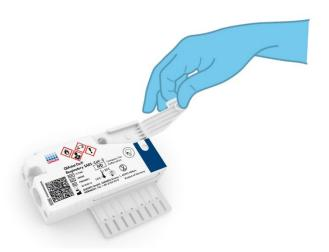
Figure 6. Opening the sample lid of main port.
