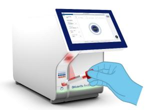
Figure 11. Scanning sample ID bar code.
