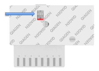
Figure 3. Sample inspection window (blue arrow).
