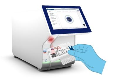
Figure 12. Scanning QIAstat-Dx Respiratory SARS-CoV-2 Panel Cartridge bar code.
