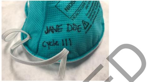
Figure 1: Chain of custody identification of N95 compatible respirators
