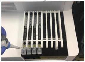
Figure 4: Adding Controls to the Cartridge
