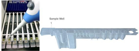
Figure 8: Test Cartridge Showing Sample Well
