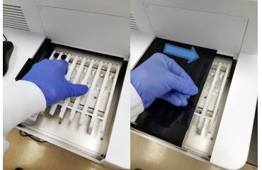
Figure 7: Inserting Rack and Closing Instrument Door
