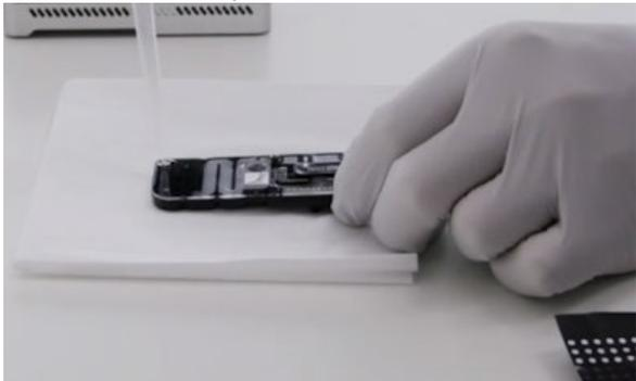
6. Return flow cell to tray. Apply the original plastic snap to close the spotON port.
