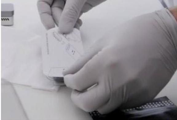
7. Place sealed flow cell tray back into pouch and close zippered pouch.
