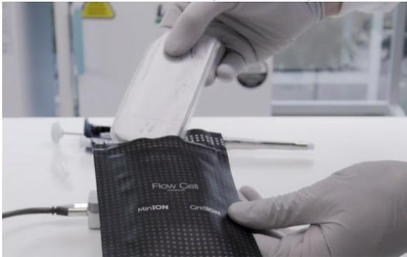
8. Store sealed, flushed Flow Cells at room temperature. Contact Clear Labs service to arrange return shipping.
