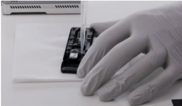
4. Close priming port by turning gate counter clockwise.
