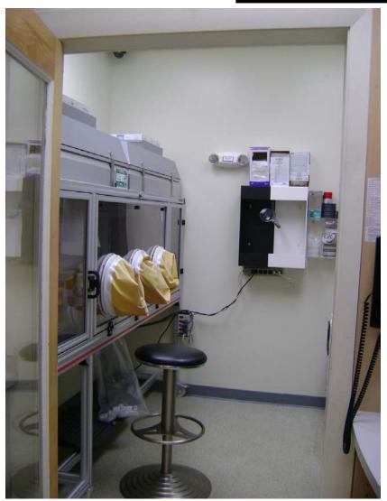
The glove box that provides ISO 5 conditions so that aseptic processing operations can occur was located in an unclassified room without HEPA filtered air.
