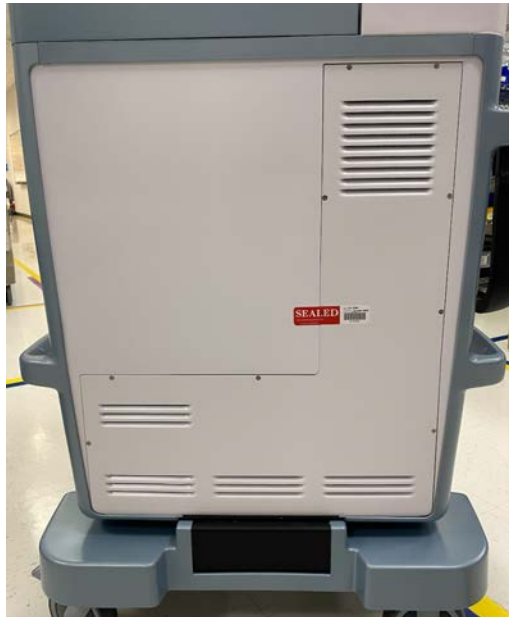
Figure 24: Photograph of Tamper Evident Seal on Console
