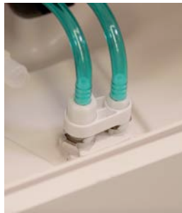
Figure 33: HPM Gas Lines Connections
