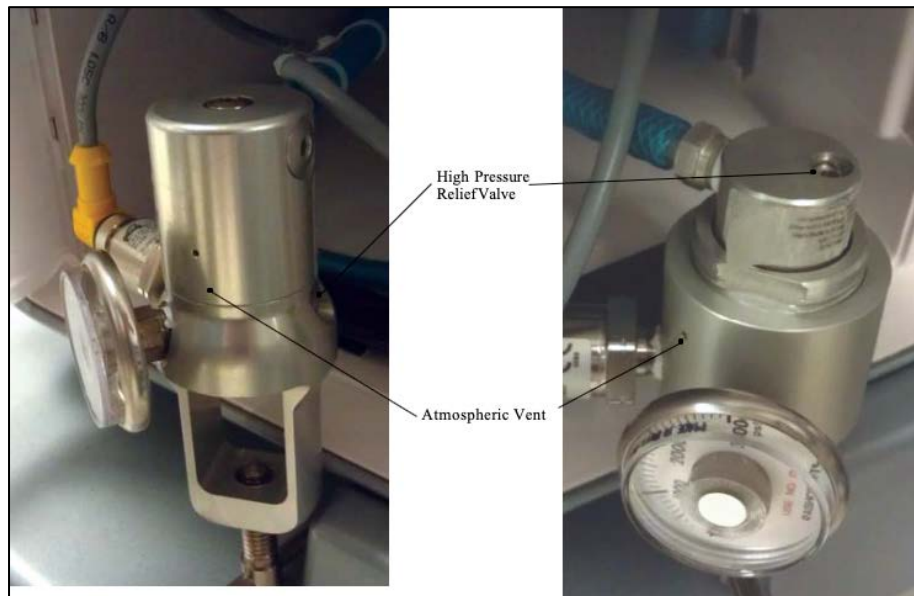
Figure 1: Left: CPI Regulator (note smooth body); Right: PI Regulator (note threaded body)
