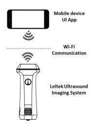
IV. The imaging system houses a built-in battery, multichannel beamformer, prescan converter and Wi-Fi components
